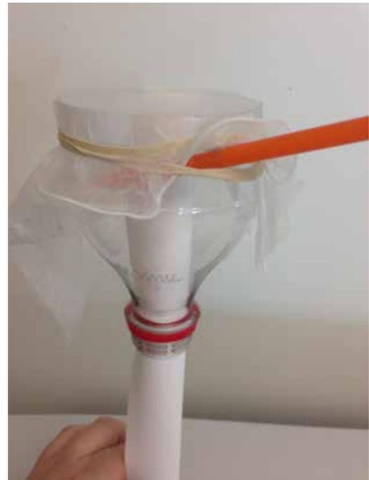
Lastly, insert the drinking straw through the hole you punched. When you blow through the straw, your breath increases the pressure in the bottle, causing the membrane to rise. When this happens, the air is forced down the paper tube, and the membrane returns to its original position. As you continue to blow air through the straw, the membrane will vibrate quickly, which will cause sound!
